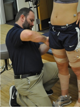
Placement of reflective markers on the torso and legs during setup
