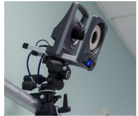
Infrared camera that detects the reflective markers placed specific places on your joints
